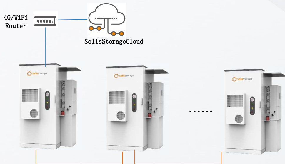
Up to 10 PrimePower connected in parallel mode on AC side
